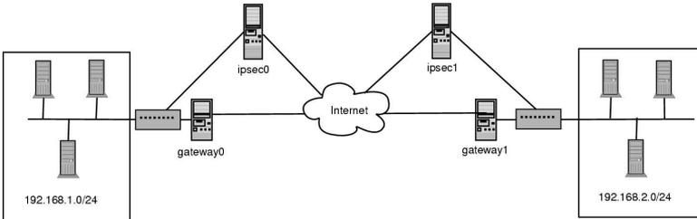
**Figure 6-1. A Network-to-network IPsec tunneled connection**
